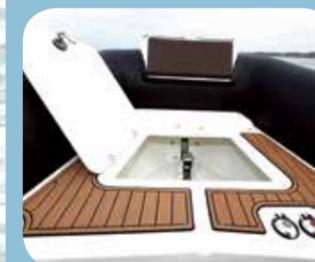
The anchor locker houses a windlass feeding through the stem.
